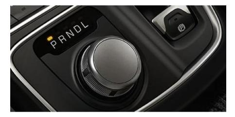
The all-new nine-speed automatic transmission includes a Rotary E-shift. The Rotary E-shift features a wide gear ratio spread that provides smooth, indecipherable transfer between gears and efficiency in all gears and speeds. It operates electronically rather than mechanically, requiring less interior space for components. The Chrysler 200 is the only car in the segment to offer a nine-speed automatic transmission<sup>+</sup>.
