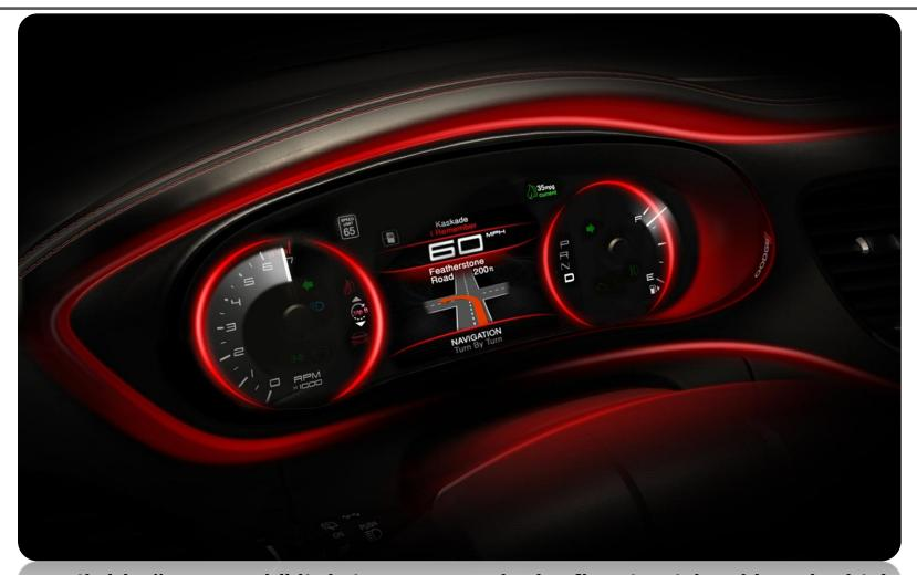
Available "racetrack" lighting surrounds the floating island bezel which houses the segment-exclusive 7-inch Thin Film Transistor (TFT) customizable gauge cluster display with light pipe surround.
