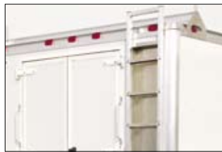
Rear access ladder allows easy access to aluminum ladder rack.
