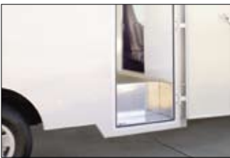
Ultra-low Step Saver side swing door with low step well and low-height cab access door for easy access.
