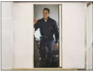
Top Hat cab with full-height cab access door lets a driver comfortably stand up and conveniently walk into the cargo area.
