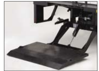
Tuck away lift gate eases loading of bulky or cumbersome cargo.
