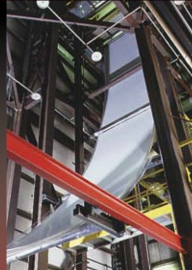
FRP being produced at Supreme's Tower Laminating plant in Ligonier, IN.
