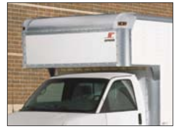
Cab-over attic extension increases cargo storage space.
