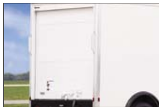
Full-width, roll-up rear door with side seals for easy access in tight delivery spaces.
