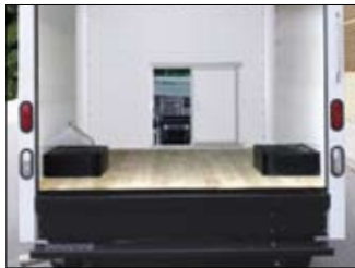
Wheel boxes and steel skirting provide for a lower front floor.
