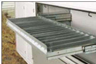
A horizontal roll-out shelf offers 21 adjustable bin spaces for small parts and tools.
