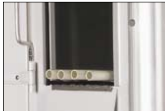
Specially designed rear pipe door simplifies loading and unloading.
