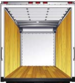
Standard: 3/8" plywood lining full-height side walls.
