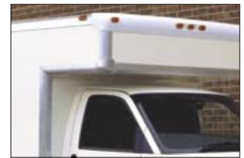
Cab-over attic for increased cargo storage capacity.
