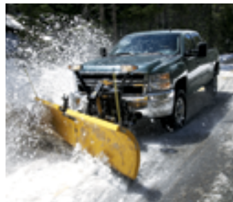
Every HD 4x4 model can accommodate a snow plow with the available Snow Plow Prep Package, thanks to massive forged upper control arms and a Front Gross Axle Weight Rating of up to 2722 kg (6000 lb.).
