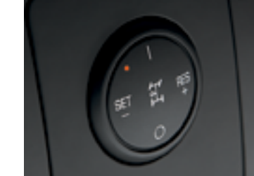
Power Take-Off (PTO) capability 5 allows HD Chassis Cab, with the available Duramax 6.6L V8 Turbo-Diesel engine, to power auxiliary equipment like a dump body or hydraulic motors for generators and tools. This feature runs off the available Allison 1000 Series 6-speed automatic transmission.
