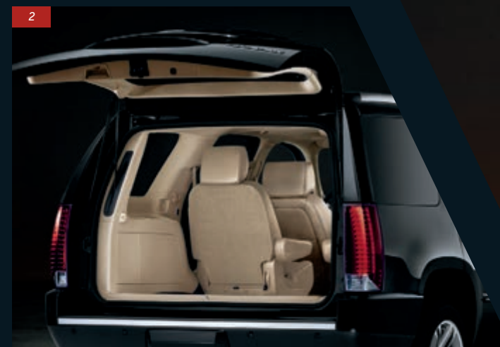
2 The standard power liftgate can be opened or closed by pressing a button on the key fob. Additional switches are located on the instrument panel and in the cargo area.
