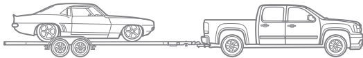
SIERRA HYBRID CREW CAB 2WD 5.3L V-8 VVT 6000 LBS (MAX) TRAILERING CAPACITY 1
