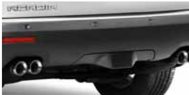
FIGURE 3: MOLDED TRAILER HITCH CLOSEOUT
