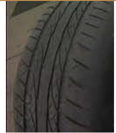
Irregular wear due to lack of regular tire rotations
