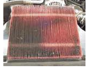
Dirty and restricted air filter
