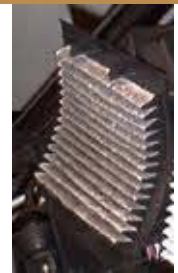
A dirty and clogged cabin air filter
